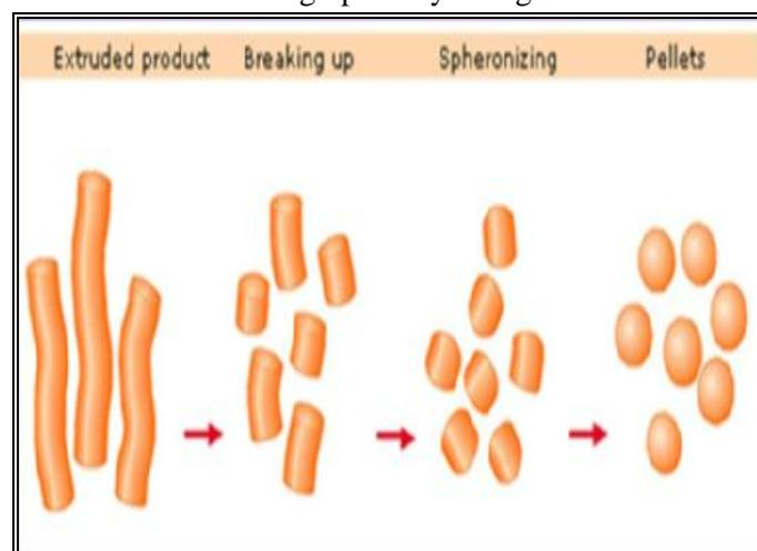
**Fig 4. Extruded product spheronizing process.**
