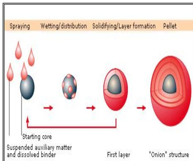
**Fig 2. Principle of the solution and suspension layering process.**
