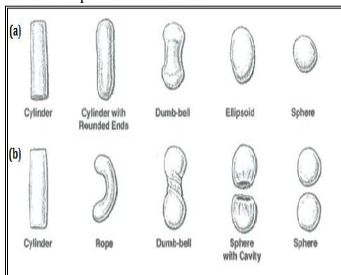
**Fig 9. Schematic representation of different pellet formation stages during spheronization.**
