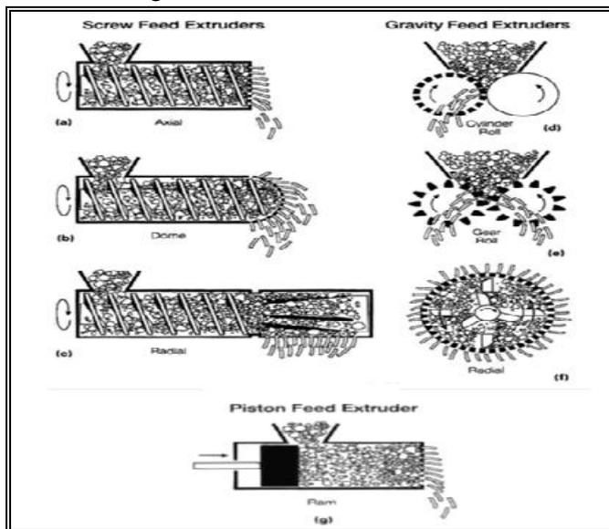
Fig 7. Schematic diagram of extruder types used in extrusion/spheronization: screw feed (a. axial-, b. dome- and c. radial- type), gravity feed (d. cylinder, e. gear and f. radial- type) and piston feed (g. ram) extruders.
