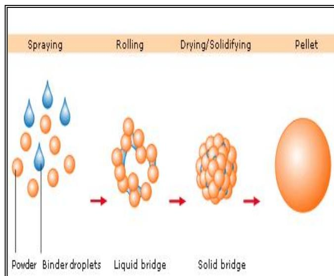
**Fig 3. Principle of the direct pelletization process.**
