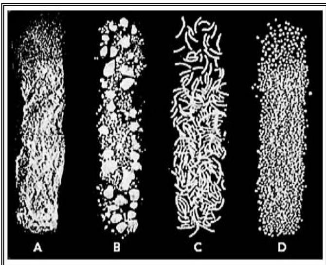
Fig 6. Product produced by the first four extrusion/spheronization process steps: (a) powder from dry mixing, (b) granules from granulation, (c) extrudate from extrusion, and (d) spheres (pellets) from spheronization.
