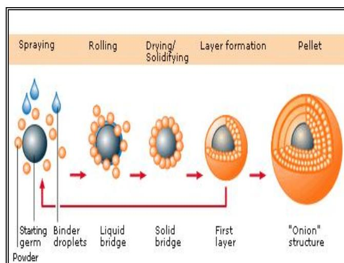
Fig 1. Principle of the powder layering process.
