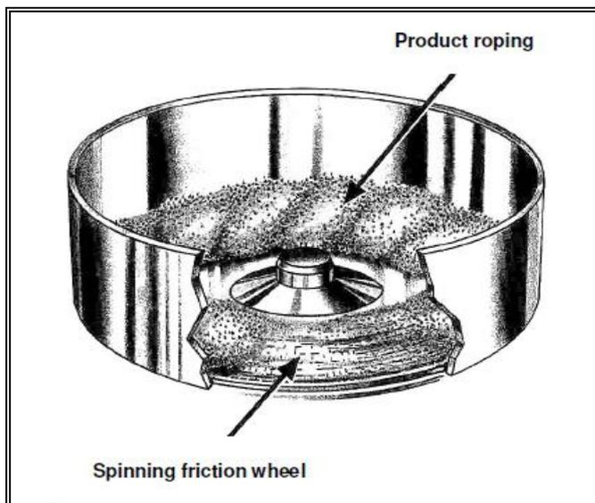
Fig 8. Schematic representation of the "rope-like" motion during spheronization.
