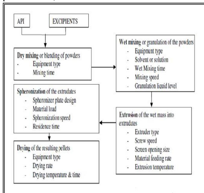
**Fig 5. Extrusion/spheronization process flow chart with individual processing variables.**
