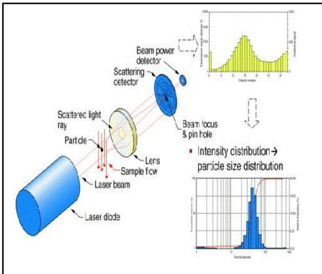
**Fig 9. Working Principle of instrument for particle size analysis.**
